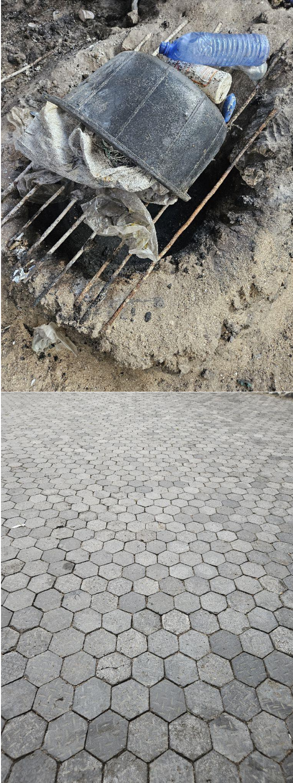
Photo 12: Plastic processing, paving stones, RDG, Goma, DRC Photo13: Recycled plastic paving stones, RDG, Goma, DRC
